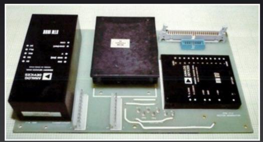
8 Channel AC/DC Ground Fault Measurement
