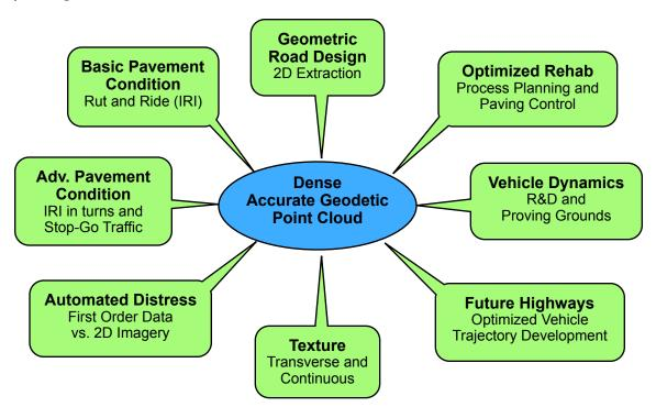
**Basic Pavement Condition** calculations for Rut and Ride were implemented by PSI by 2004. The Ride module supports up two 32 longitudinal profiles as user specified offsets. The Rut module provides options for all the modern rut algorithms as well as the 3 and 5 point methods for grandfather purposes. PPS customers have and continue to implement there own post-processing more directly integrated to there Pavement Management Systems (PMS) design.
