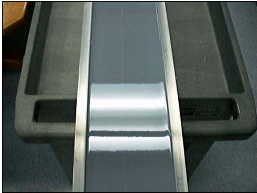
Figure 5. Finished shiny epoxy surface on calibration beam reflecting the overhead florescent lighting fixture.
