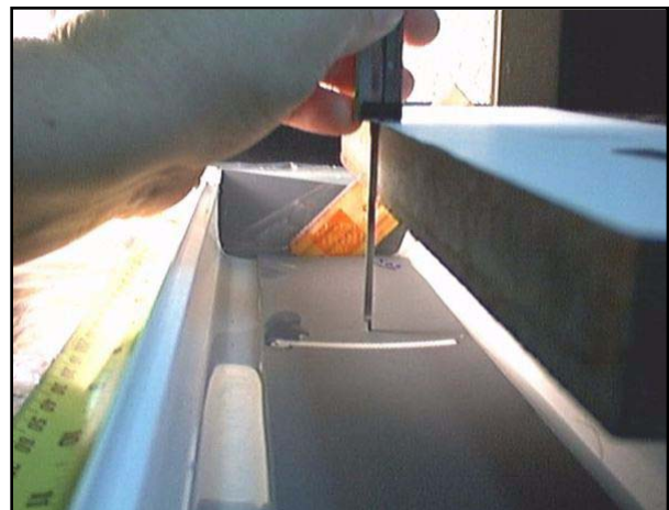
Figure 2. Profiling mylar surface with caliper and elevated reference plane established by a board.
