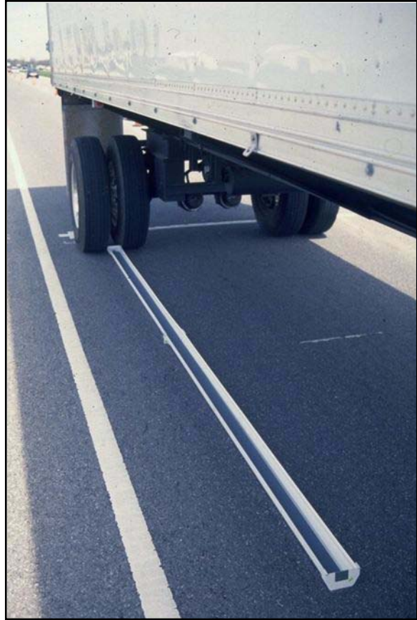
Figure 3. Water trough calibration surface under RWD trailer.
