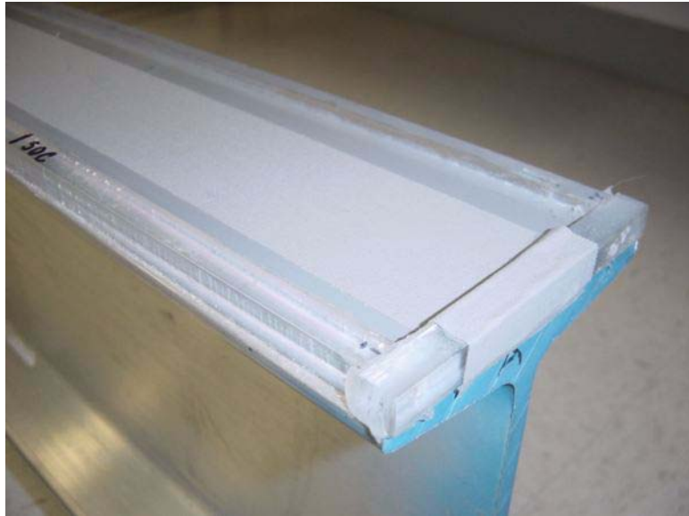
Figure 6. Tape covering epoxy on calibration beam.
