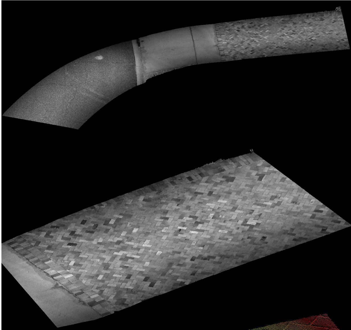
The top two images are lidar return displayed as gray scale. They are not images produced by a camera system. The lower image is color coded elevation.
